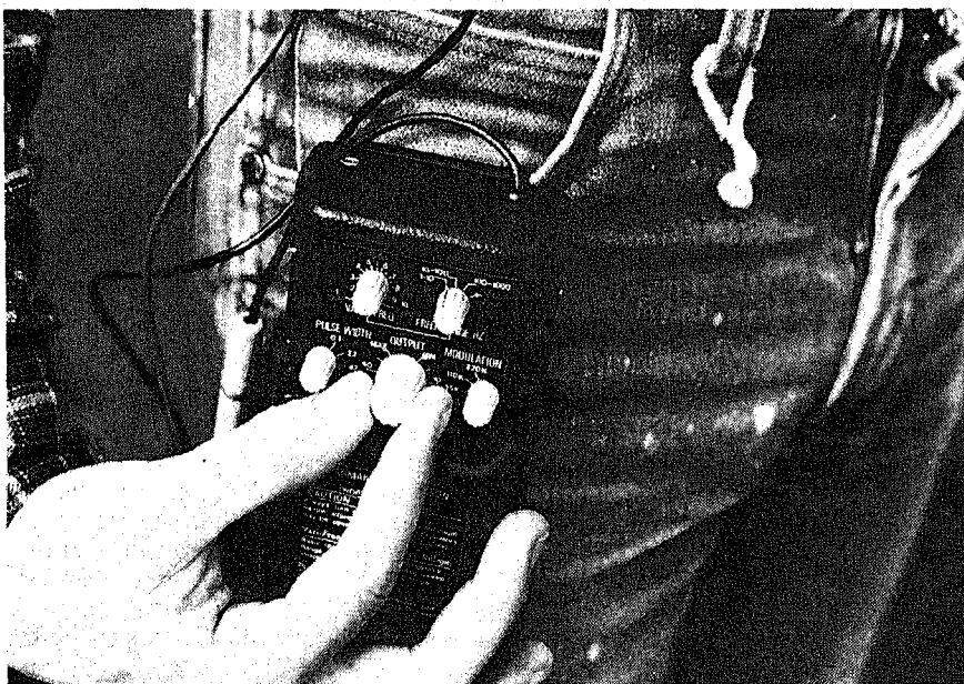
Fig 3. The Pharmakon-Patterson Stimulator, showing the patient adjusting the voltage (output). All the other settings are controlled by the therapist
